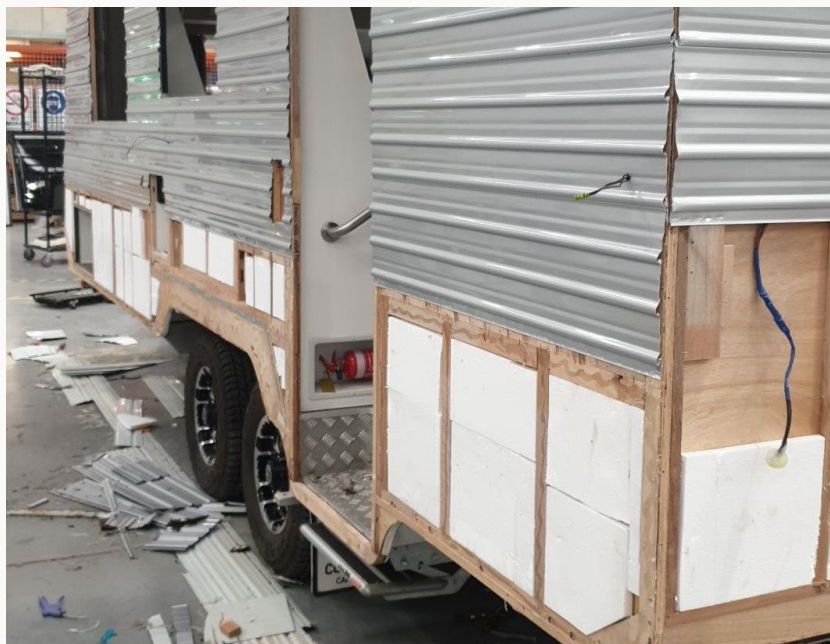
Figure 15 Stick and tin wall construction (2020) by Caravan Fix Rockhampton https://www.caravanfix.com.au/location/caravan-repairs-
