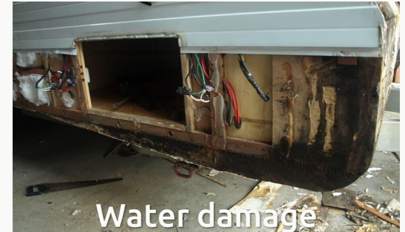
Figure 18 Water damage due to poor quality (2020) by P. Lord ( https://www.caravancampingsales.com.au/editorial/details/lemon-caravans-and-the-law-122225/ )
