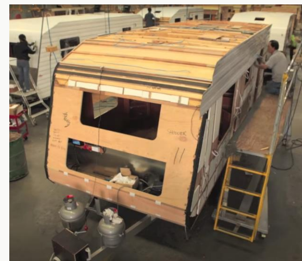
Figure 24 Styrene insulation in walls and aluminium cladding added (2022) by Concept Caravans http://y2u.be/mHluQGHCxp0
