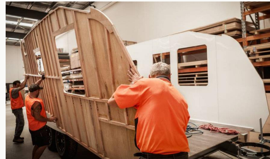
Figure 22 Standard Timber wall construction by CaravansPlus (2020) https://www.caravansplus.com.au/guides/self-build-guide-5-floor-wall-and-roof-construction-a-122.html
