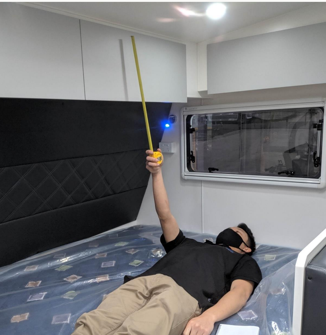
Figure 10 measuring head clearance space
