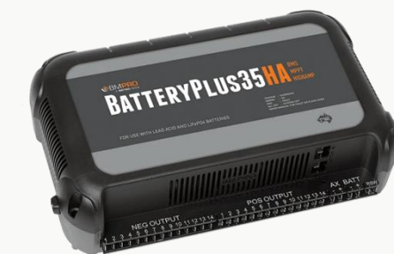
Figure 23 Batteryplus battery management system with solar regulator (2021) by BMPRO
